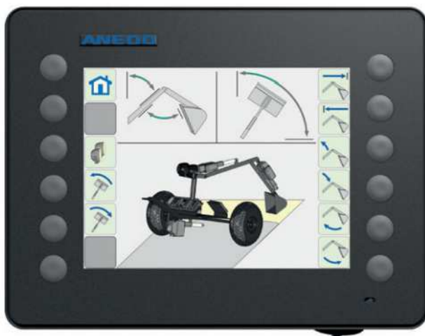
Figure 14: Iso 1 Box compact operator terminal with full ISOBUS functionality
