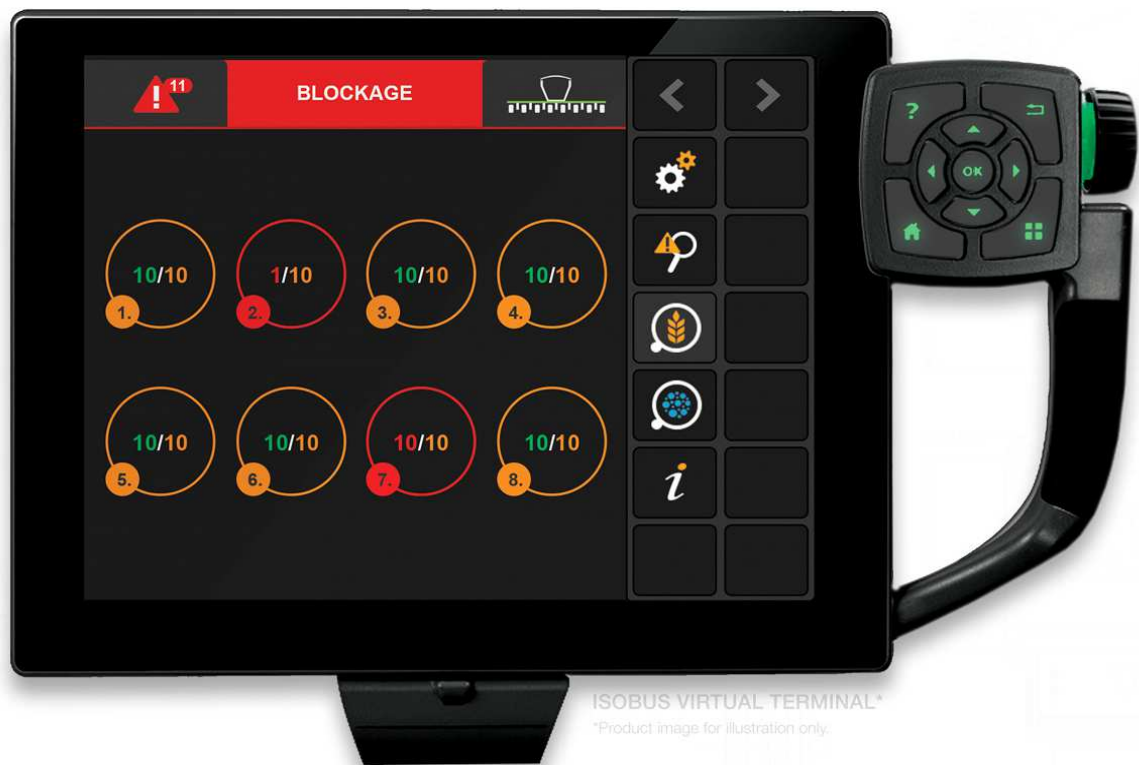
Figure 1: ISOBUS controlling displayed by the tractor's universal terminal
