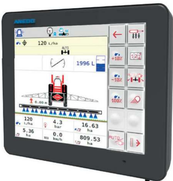
Figure 16: Iso 2 Box: 8,4" touchscreen with SlideStick technology
